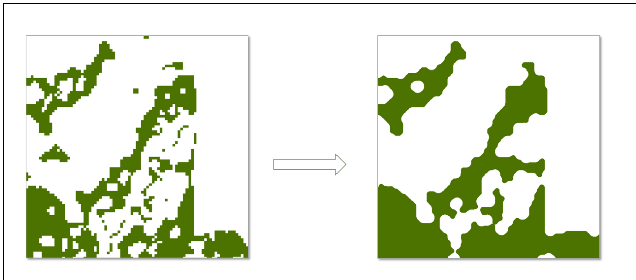
Figure 4. An example of spatial arrangement of input data for and results of the stand identification process converting RS-FRIS grid data into stand polygons.
